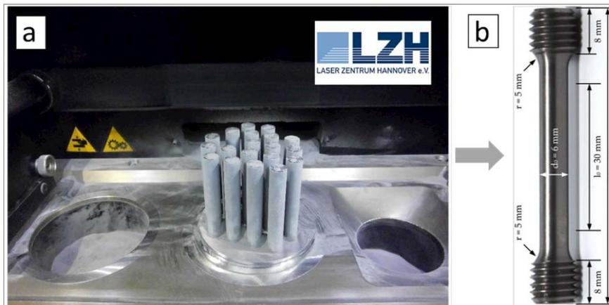
Figure 12. Tensile test set of Ti-42Nb PBF-LB built specimens fabricated by Laser Zentrum Hannover
