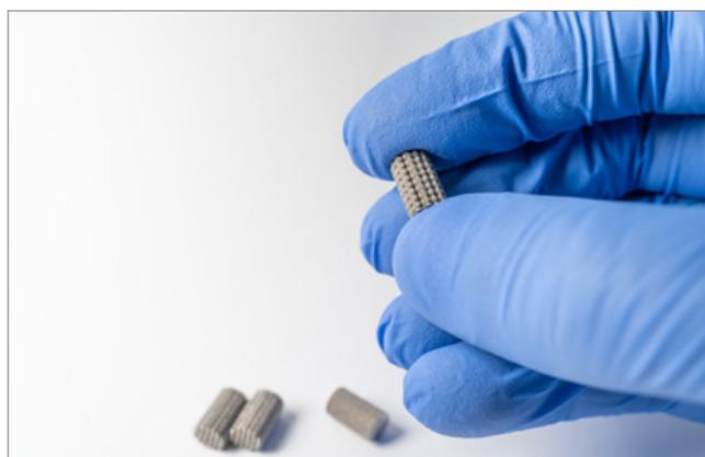
The winning paper analysed the properties of solid and lattice structures made of Ti-25Ta alloy (Photo: N.Soro)
