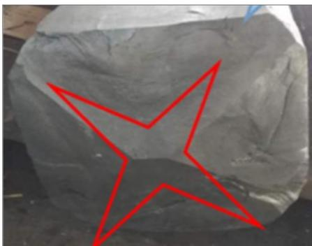
Figure 5: Deformation section of conventional forging
