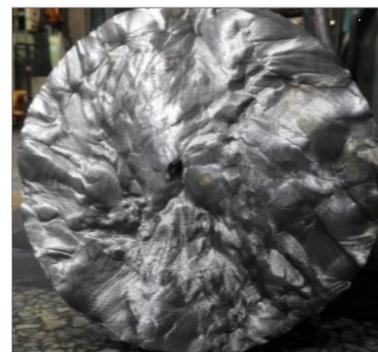
Figure 6: Deformation section of die SPD forging
